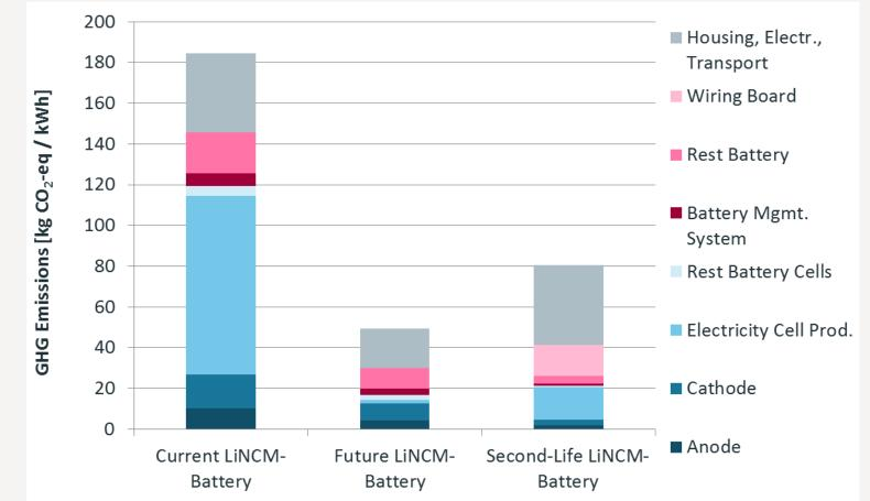
Electricity demand of cell production contributes about 50% to GHG emissions of current batteries
