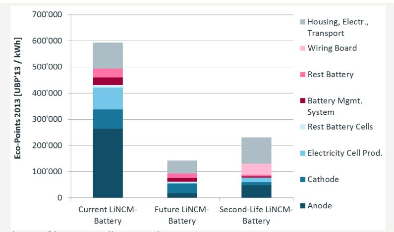
Share of battery cells in total impacts: current batteries: 70%, future batteries: 40%, second-life batteries: 30%
