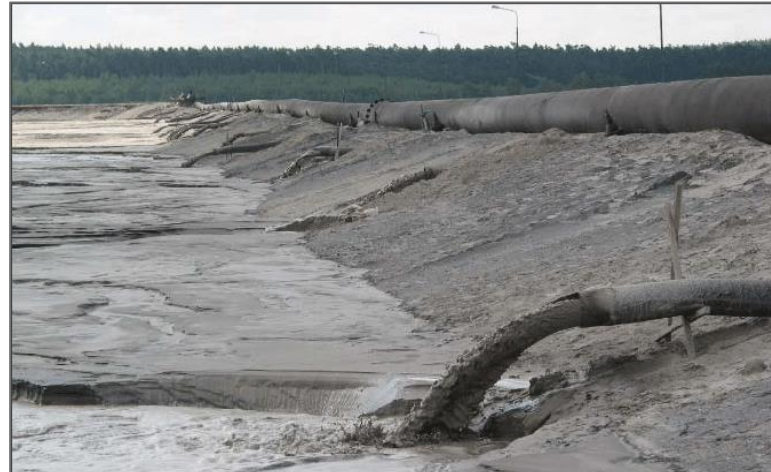
Tailings: Materials left after the process of separating valuable fractions from the ores
